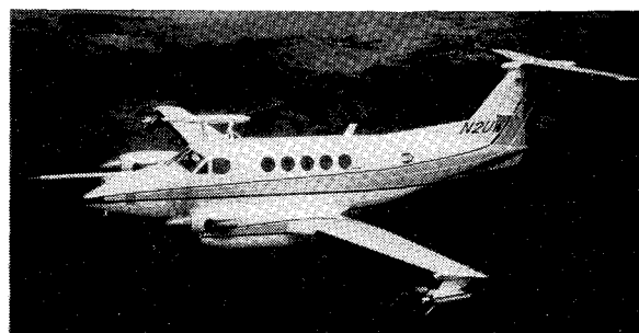
Fig 1 Research airplane N2UW as modified with wing tip pylons, decelerator (tube on top), and noseboom.
